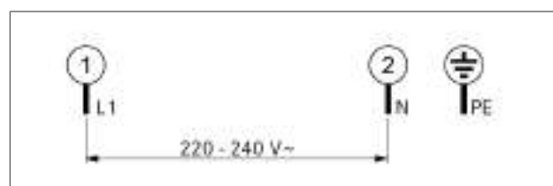
Fig. 4.86 1-phase connection diagram
